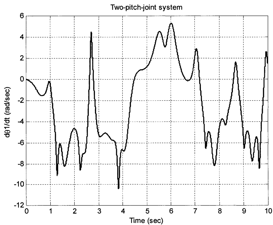
Figure 3.25 1 st joint angular velocity versus time at the initial condition: \tau_1 = 1, \tau_2 = 1, \underline{z}_0 = \underline{0}
